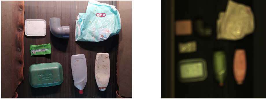
Fig. 3: Indicative snapshot of the experimental procedure. The left image shows the arrangement of 7 recyclables (plastic categories PP, PVC, LDPE, OTHERS, PS, PET, HDPE) using an ordinary RGB representation. The right image shows the pseudo-colored raw image captured by the hyperspectral camera Specim FX17e.
