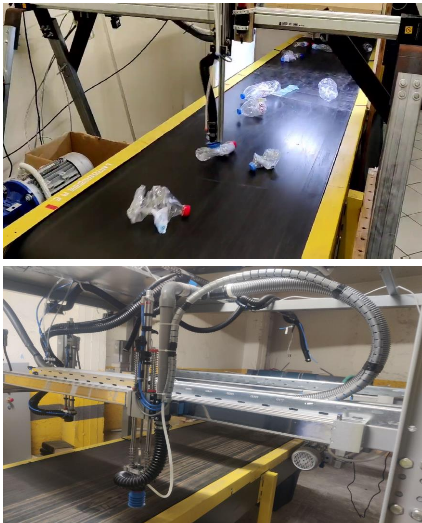
Figure 14. Two different versions of the 1.5 DoF RoReWo.
