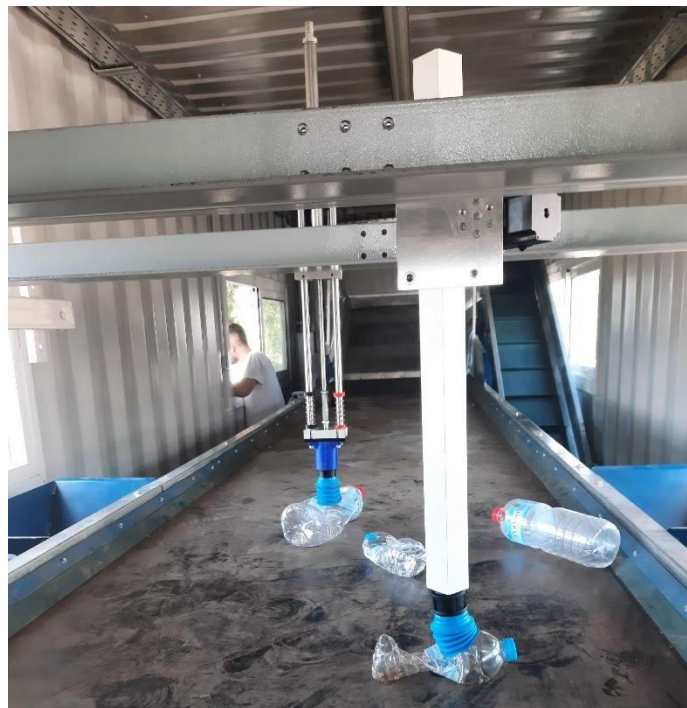
Figure 27. The first 1.5DoF RoReWos being installed inside the prMRF.
