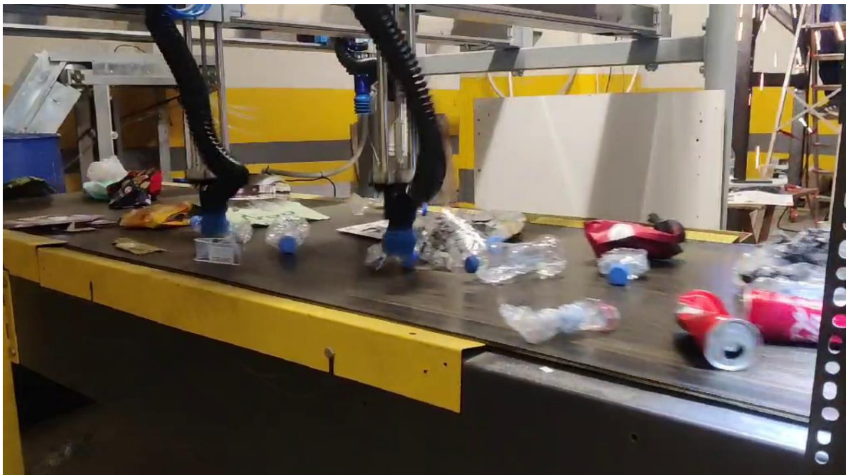
Figure 26. A snapshot of a three RoReWo-Team working on PET recovery.
