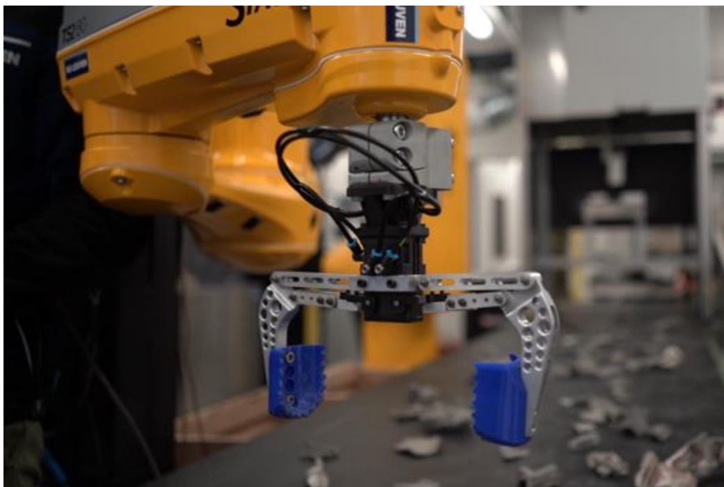
Figure 17. Pneumatically actuated parallel gripper.
