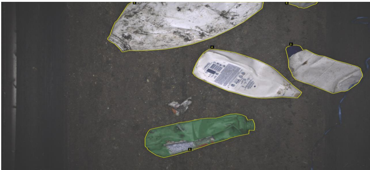
Figure 9: Annotated RGB image: isolated waste stream with HDPE objects annotated.
