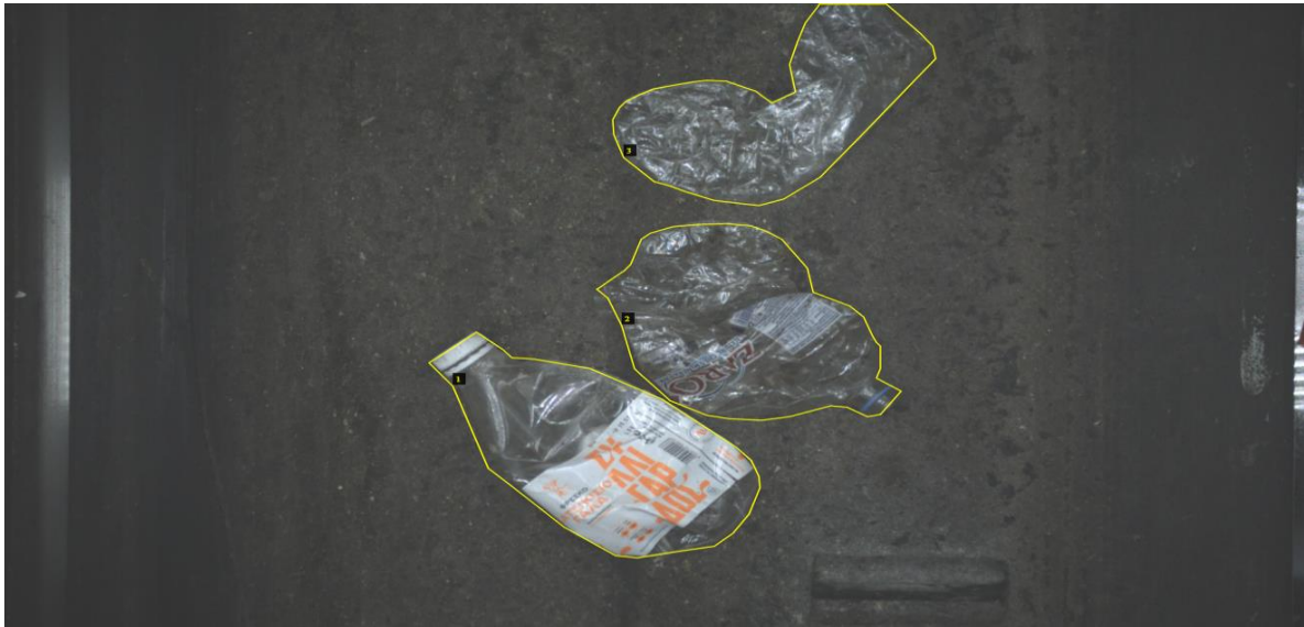
Figure 8: Annotated RGB image: isolated waste stream with PET objects annotated.
