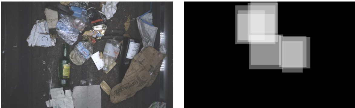
Fig. 13: Overlaid binary classification maps, resulting in an average, probabilistic map of PET items in the reference image.
