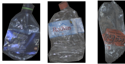
Fig. 1: A sample of object-images extracted from industrial belt-images.
