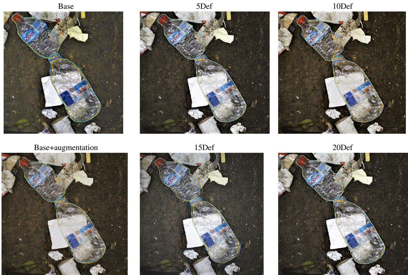
Fig. 6: Indicative identification of PETE bottles by the models trained with the different datasets considered in the current work. All images are zoomed to facilitate visual inspection. In all images model prediction polygon is shown in orange and groundtruth polygon is shown in blue.
