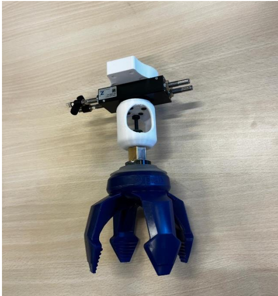
Piab Pi-Grip fingers mounted on a Zimmer swivel actuator.
