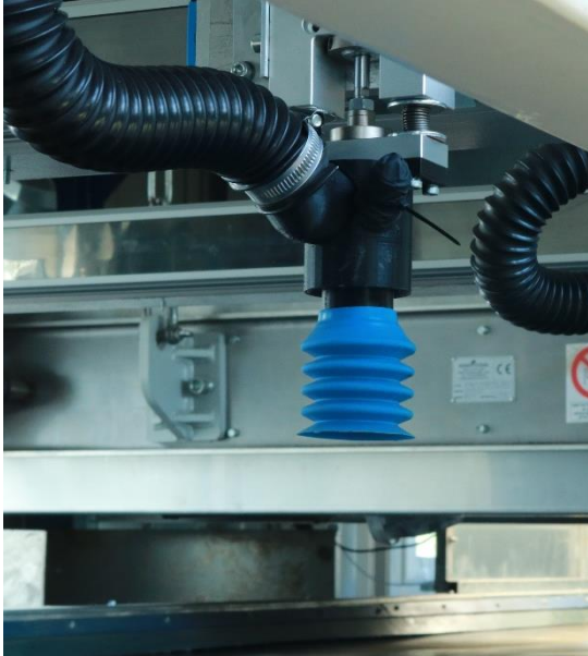
Suction cup gripper with blower generated vacuum installed in the Reclaim Pr-MRF
