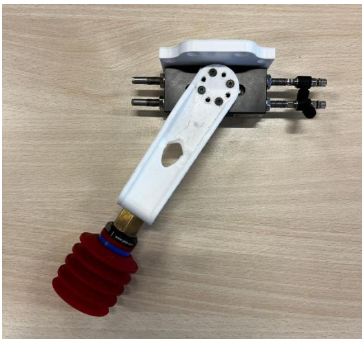
Piab suction cup installed on a swivel arm powered by a Zimmer swivel actuator.
