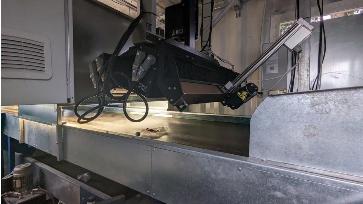
Fig. 1: The adapted Visum HSI™ hyperspectral imaging system with its lights mounted front and back (side view)
