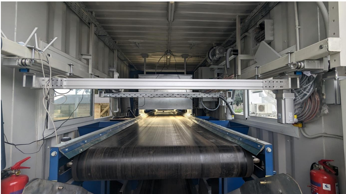
Fig. 3: The second section after the magnet of the prMRF with RGB camera box with lights and the two linear 3 DOF (first from the camera box) and the 2.5 DOF (the second one).
