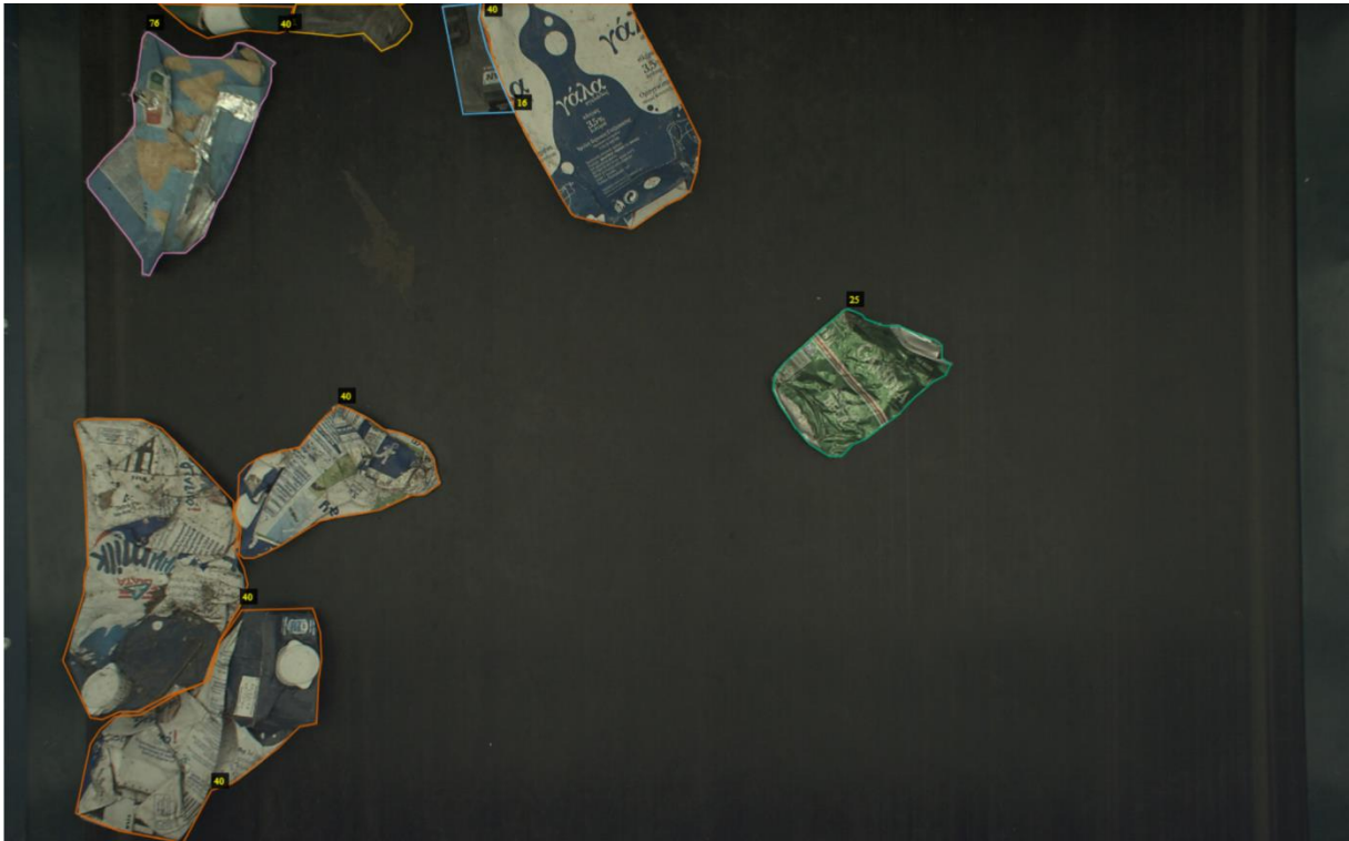
Fig. 10: Annotated RGB image: mixed waste stream with PET, Aluminum, Tetrapak and Other objects annotated.
