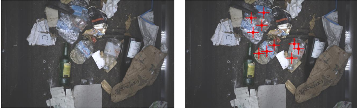
Fig. 9: Reference Image, where the users are asked to indicate the centre of PET items, and indicative input of multiple users, as shown in the RDG.
