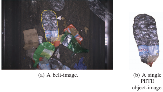
Fig. 1: An example of a belt-image taken in the MRF (left) and a segmented PETE object-image (right).
