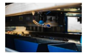
The RECLAIM solution uses multiple robots with modular grippers to efficiently pick and handle different types of waste, depending on their composition. Additionally, Al-driven computer vision can accurately identify waste, allowing robots to maximise sorting effectiveness. Packed inside a portable container, these innovations will significantly enhance local-scale material recovery activities with industrial-level efficiency for a Circular Economy in European islands and remote tourist areas.
